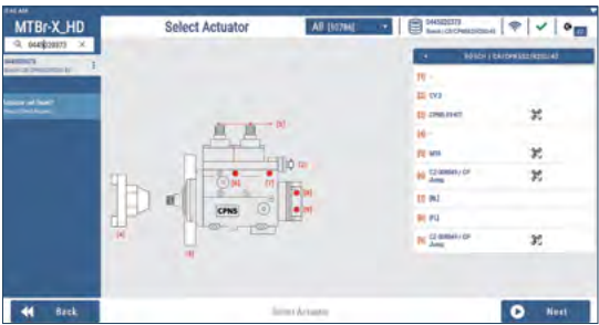
Every connection, mapped on screen: numbered points, exact part numbers and adapters for each component, mount, connect and test with zero guesswork.
